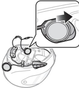
**[Once installed, the position of the speaker unit can be adjusted to rider's ear position]**
