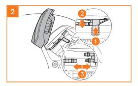
**Note:** When you need to un-plug the connector, please wiggle and pull it. It will help the connector connection be released more easily.
