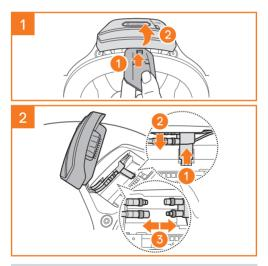
Note: When you need to un-plug the connectors, please wiggle and pull them. It will help the connector connection be released more easily.
