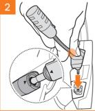
Install the microphone by pressing firmly on the area marked with the orange circle.
