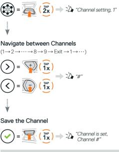
Note: To exit the Channel Setting, tap the (+) Button or (-) Button until you hear a voice prompt, "Exit", and tap the Center Button.
