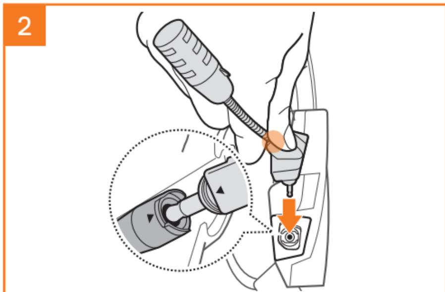
Install the microphone by pressing firmly on the area marked with the orange circle.
