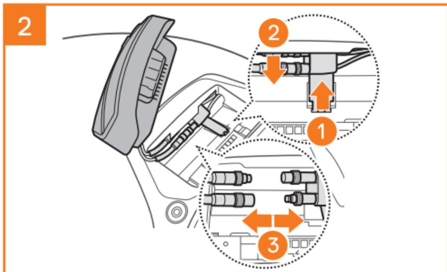
**Note:** When you need to un-plug the connectors, please wiggle and pull them. It will help the connector connection be released more easily.
