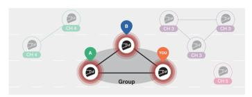
Users (You, A, and B) enter the mesh grouping by pressing the Mesh Intercom button for 5 seconds while staying in the open mesh. They don't need to be on the same open mesh channel to create a group mesh together.
